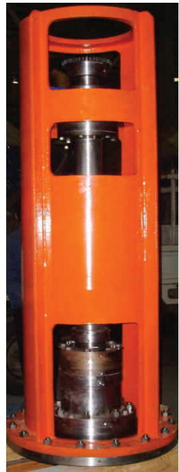
为大震锅炉生产的搅拌密封传动装置 The Agitator Drive transmission device for TAIJUNE BOILER company
